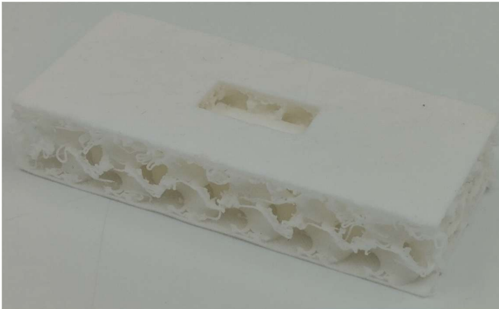
Figure 4: Low infill degrades the printing quality
